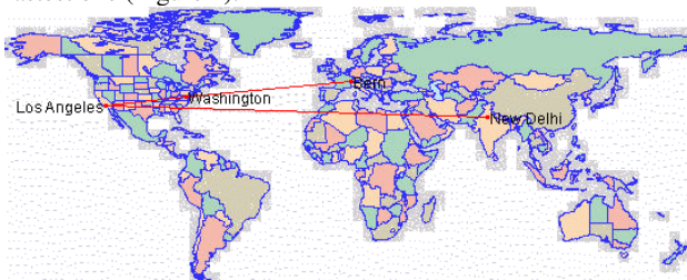
Figure 4: A graphical trace-route of a Internet path covered between a server in Switzerland and the server hosting ISPRS Commission 7 in India. The request passes through US as faster route compared to a Middle East route. Source: [VisualRoute].
