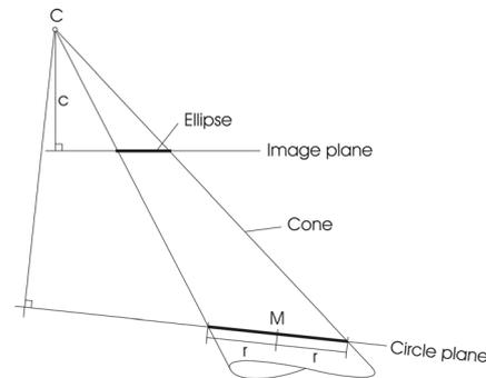
Figure 7: View cone which touches circular target.
