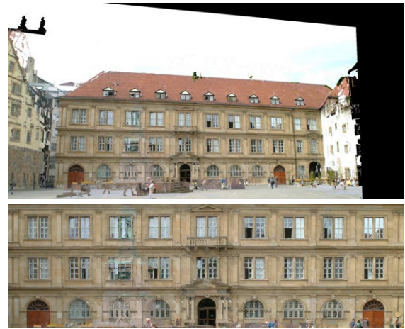
Figure 9: The result of the image fusion with the input images shown in figure 8. The bottom picture shows the final rectification onto the façade's rectangle. The statue has completely disappeared and most of the pedestrians were suppressed. The bottom picture shows the final rectification onto the façade's rectangle. Note the improvement to each of the rectified images in figure 8.
