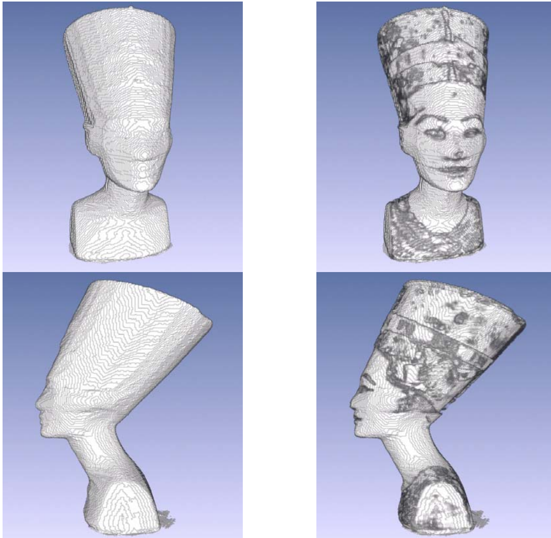
Figure 10: Different viewpoints of the Nefertiti cube. The result of shape from silhouette (left), refinement by voting based carving (right)
