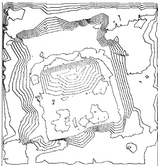
Fig. 12. Segmented disparity map from 4K matching
