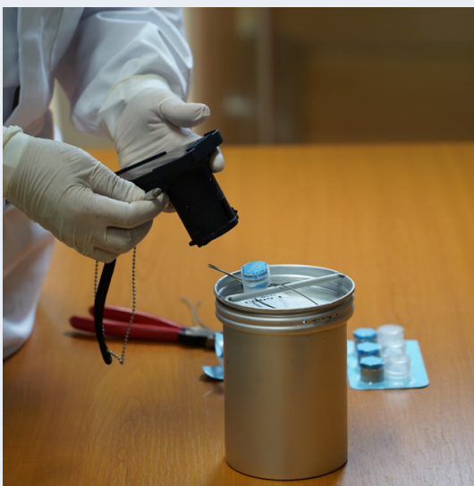
An IAEA safeguards inspector applying a Field Verifiable Passive Seal (FVPS).
