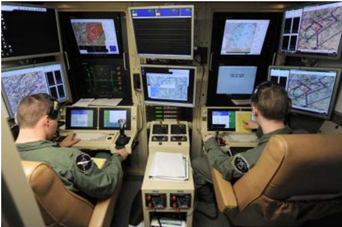
Figure 5: MQ-9 Ground Control Station
