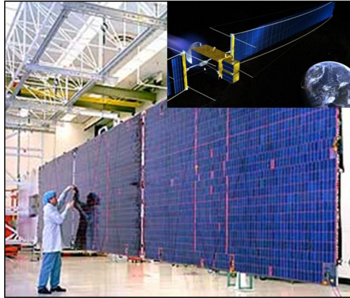
Figure 3.2: High Power Solar Array (HPSA) technology. Inset: Deployed arrays in space, as with the Integrated Blanket Interconnect System (IBIS) program
