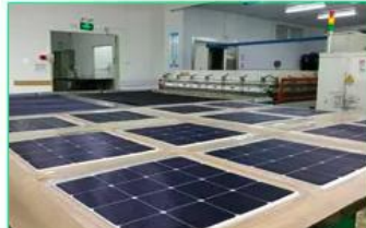
Solar panel lamination
