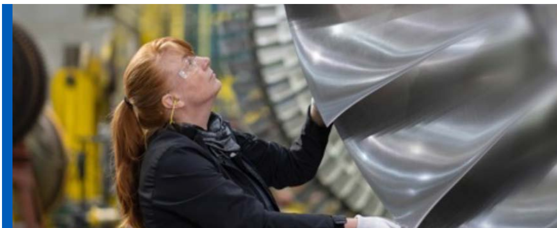
Vicki Lungford servicing a 7HA.03 gas turbine in South Carolina.
