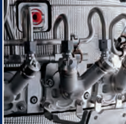
▲ The CFM LEAP has 1,001 innovations built in, including fuel nozzles with additively manufactured tips, reducing part count from about 20 pieces to one.
