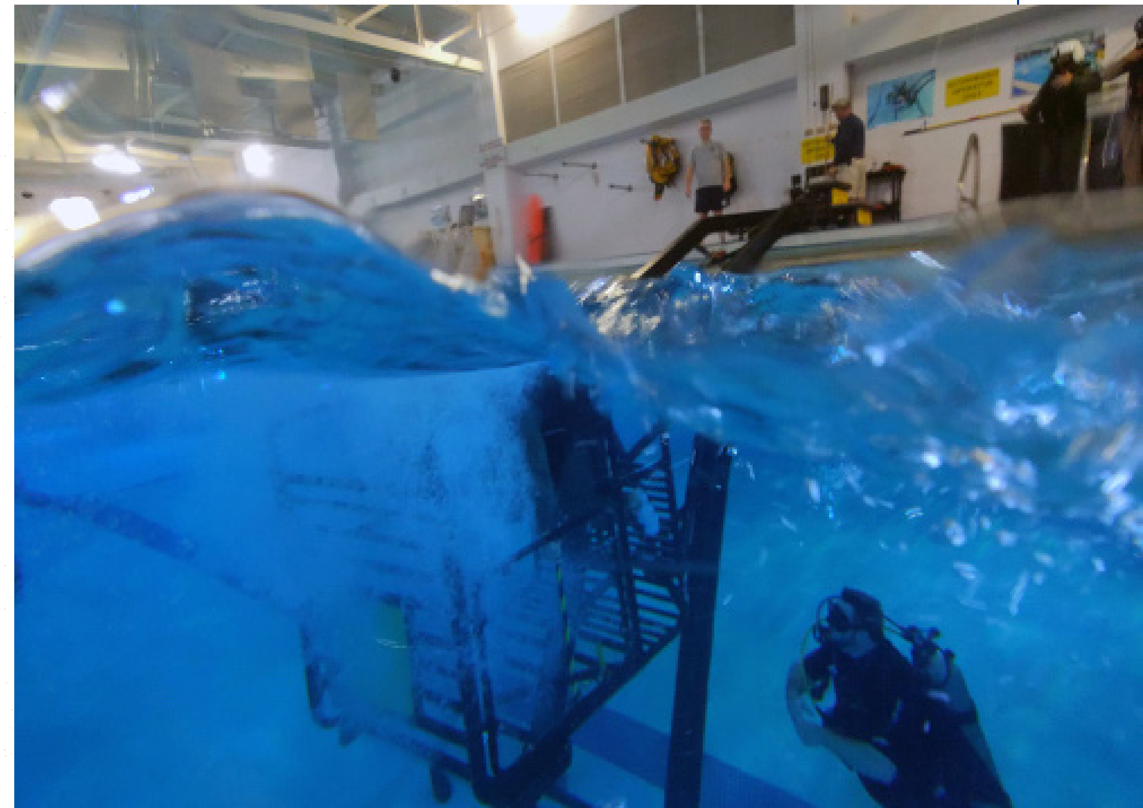
Marine Training Branch trained professionals observe Law Enforcement Officers of the Customs and Border Protection Air and Marine Basic Training Program participate in the Underwater Egress Trainer (UWET), which provides LEOs the chance to experience a submerged emergency exit from a vehicle/cockpit, on Nov. 7, 2020 at Glynco, Ga. (FLETC OPA/Brandon Spragins)
