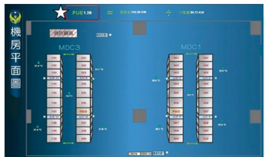
Monitoring of the Environment of the Data Handling Room (Power Usage Effectiveness (PUE) Indicator <math>< 1.3</math>, in Compliance with Green Energy Requirements)
