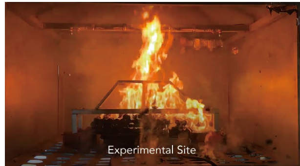
Small-scale fire experiment of electric vehicle lithium batteries
