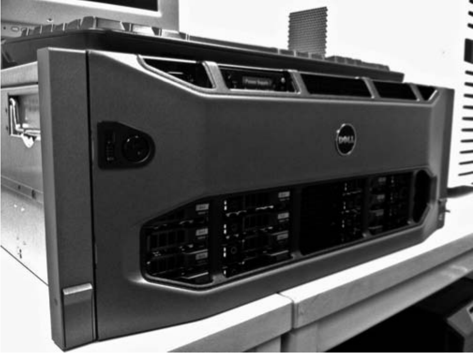
Figure 2: A commodity server capable of a combined TPC-C like transaction throughput of up to 2 million transactions per second. Notice the keyboard on top of the machine for scale.
