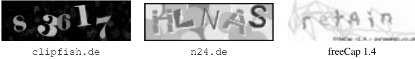
Figure 4: Careless use of color that makes segmentation and extraction of the characters trivial.
