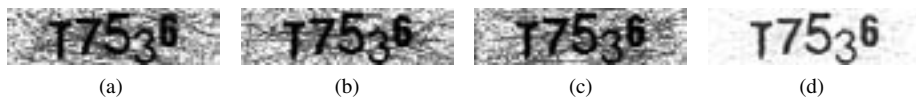
Figure 6: CAPTCHA used on quoka.de ; three versions of the same challenge (a–c) with different backgrounds. A pixel-wise multiplication eliminates background noise almost entirely (d).
