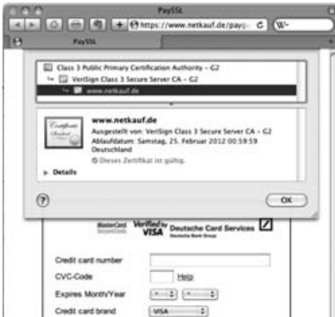
Figure 2: The “Verified by Visa” content’s <iframe> loaded into a window and the certificate information dialog of the Safari web browser
