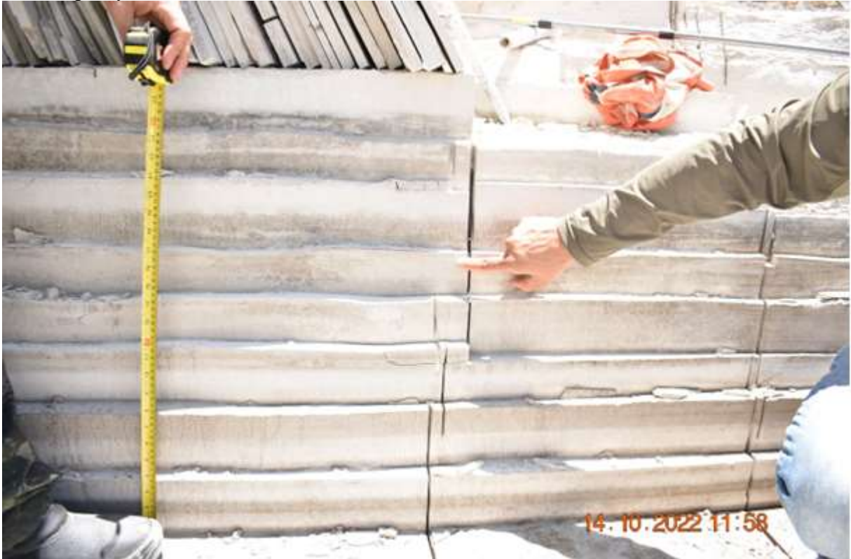
Figure 3 - Appearance of the “sete cortes” (“seven-cuts”) layer on the mining front in the Nova Olinda quarry
