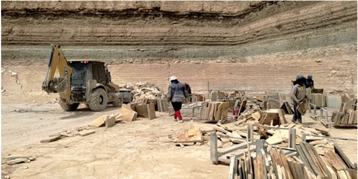
Figure 2 - Mining front of laminated limestone from the Crato Formation in the Nova Olinda quarry.
