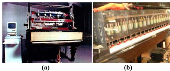
Figure 1. Trimpin’s automatic piano instruments (a) Contraption Instant Prepared Piano 71512 [30] (b) piano adaptor that strikes keys automatically.
