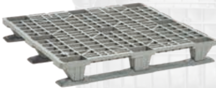
APBAS1210R Open Top Pallet On Runners D: 1200 x 1000 x 160mm W: 8.15kg Load Capacity: 1800kg Static, 1000kg Dynamic
