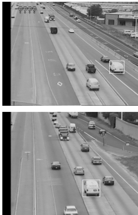
Figure 1. Images from two surveillance cameras roughly two miles apart on Highway 99 in Sacramento, California. The top image is from the upstream camera, and the bottom image is from the downstream camera. Are the two boxed vehicles the same?
