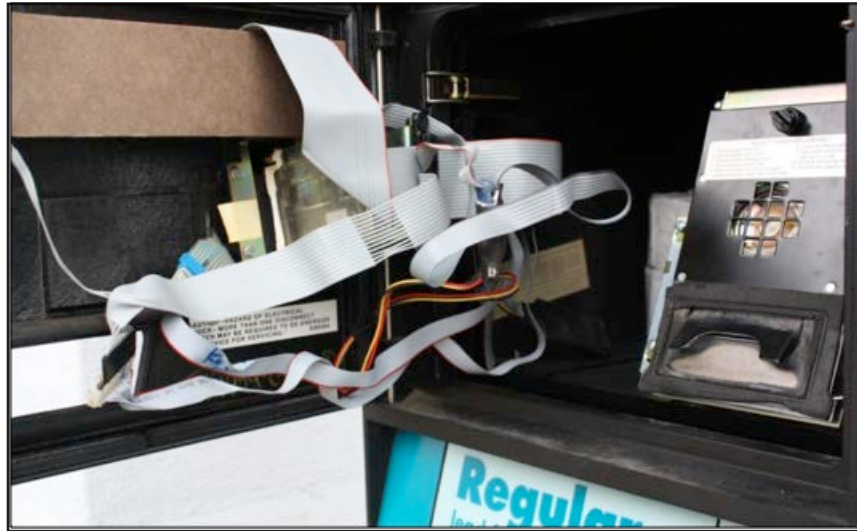
Figure 29 Skimmer Placed in a Gas Station Payment Terminal in Martinez, CA
