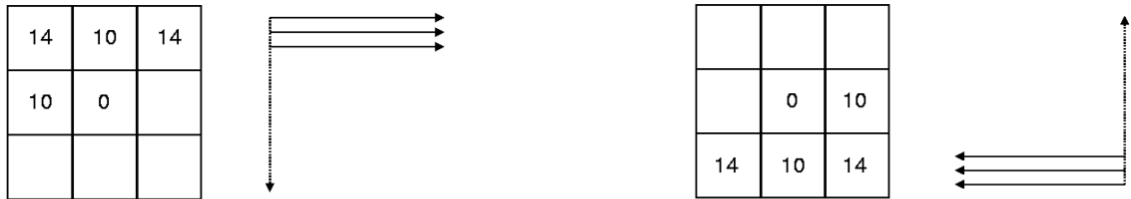
Figure 1. Templates and directions of the chamfering process used for the efficient calculation of an integer approximation to the Euclidean distance. The left template is applied row by row, top to bottom and a left to right ordering within the rows, the second template from bottom to top and from right to left.
