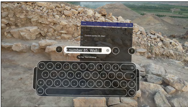
Figure 6 HoloLens note-taking app with voice recognition and keyboard entry, user view inside the headset.
