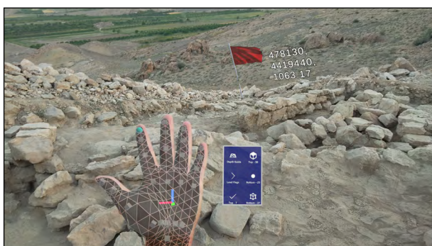
Figure 21 Placing a corner flag to set the coordinate system, HoloLens user view.
