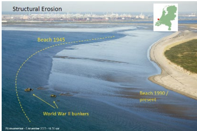
Figure 9: Coastal erosion between 1945 and 1990 in the Netherlands. Since 1990, they have been adding sand to maintain the coastline. (Source: Rijkswaterstaat)
