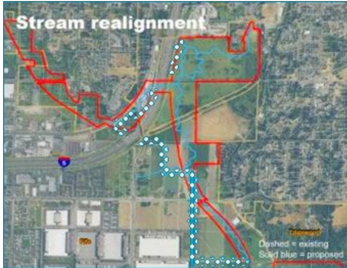
Figure 17: Planned stream realignment under the riparian restoration program. White dotted line shows existing stream location (note straight lines and right angles) while solid blue shows proposed location (note more natural meanders). (Source: WSDOT).
