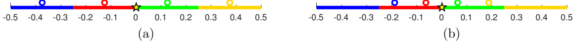
Figure 4.1: Two deployment examples in a 1-dimensional space with one FC. (a) The AC/DC two-tier quantizer. (b) The optimal quantizer. AP and FC locations are denoted by circles and star. The optimal partition cells are denoted by intervals. Each AP and its corresponding cell are illustrated by the same color.
