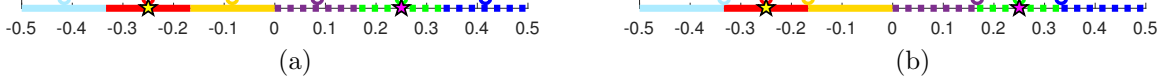
Figure 4.2: Two deployment examples in a 1-dimensional space with two FCs. (a) The AC/DC two-tier quantizer. (b) The optimal two-tier quantizer. AP and FC locations are denoted by circles and stars. The optimal partition cells are denoted by intervals. Each AP and its corresponding cell are illustrated by the same color. The two clusters are denoted by solid and dashed lines.
