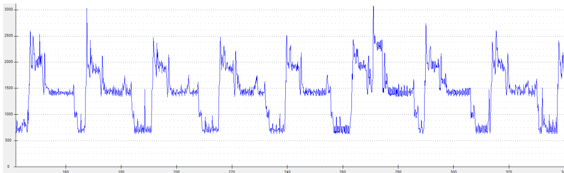
Figure 1.1. Power consumption (mW) trace of a smartphone device running six CRM applications that each periodically download a resource using the cellular radio without any form of coordination.
