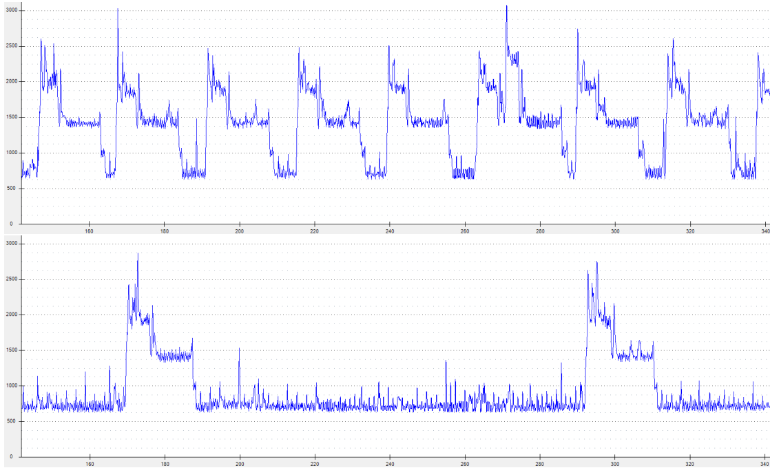
Figure 2.10. Power consumption (mW) traces from a smartphone device running a variety of naive (top) and APE enhanced (bottom) CRM applications.
