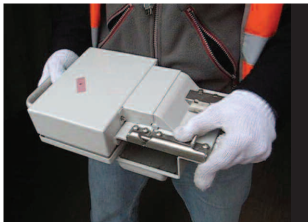
Figure 2: TREC prototype ready to be mounted on the container door. On the left is the box containing the electronics that sits within the container; at the bottom right is the antenna box that sits outside the container door.
