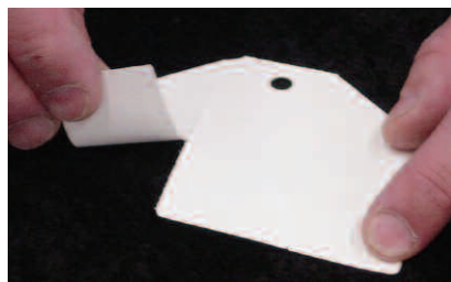
Figure 2: Partial antenna removal from a garment hang tag.
