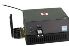
LimeNET Mini For Indoor Base Station test as "crowdcell" and as UE
