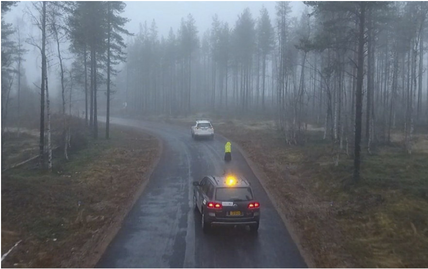
Figure 1: The 5G-assisted automated driving scenario demonstrated on the Sod5G winter vehicle test track. The front vehicle transmits LiDAR data to an obstacle detection algorithm running on a MEC server. The self-driving car Martti, behind, receives a warning and manages to go around the obstacle.
