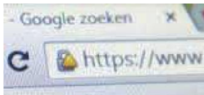
Google Chrome users receive a warning when a certificate is signed with a SHA-1 based signature issued after 2015.
