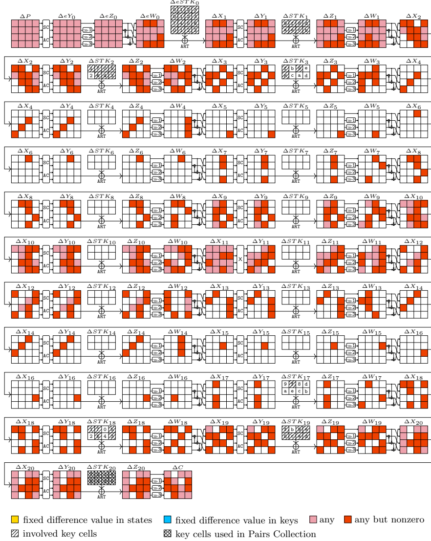
Fig. 15: The single-tweakey impossible differential attack against 21-round SKINNY-n-3n
