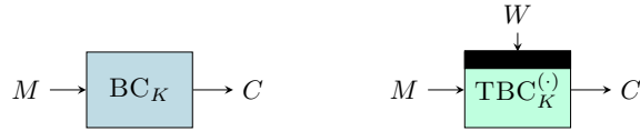
Figure 16: Block-cipher (left) and tweakable block-cipher (right). For tweakable block-ciphers, the black bar indicates that the incoming arrow ( W ) is the tweak.
