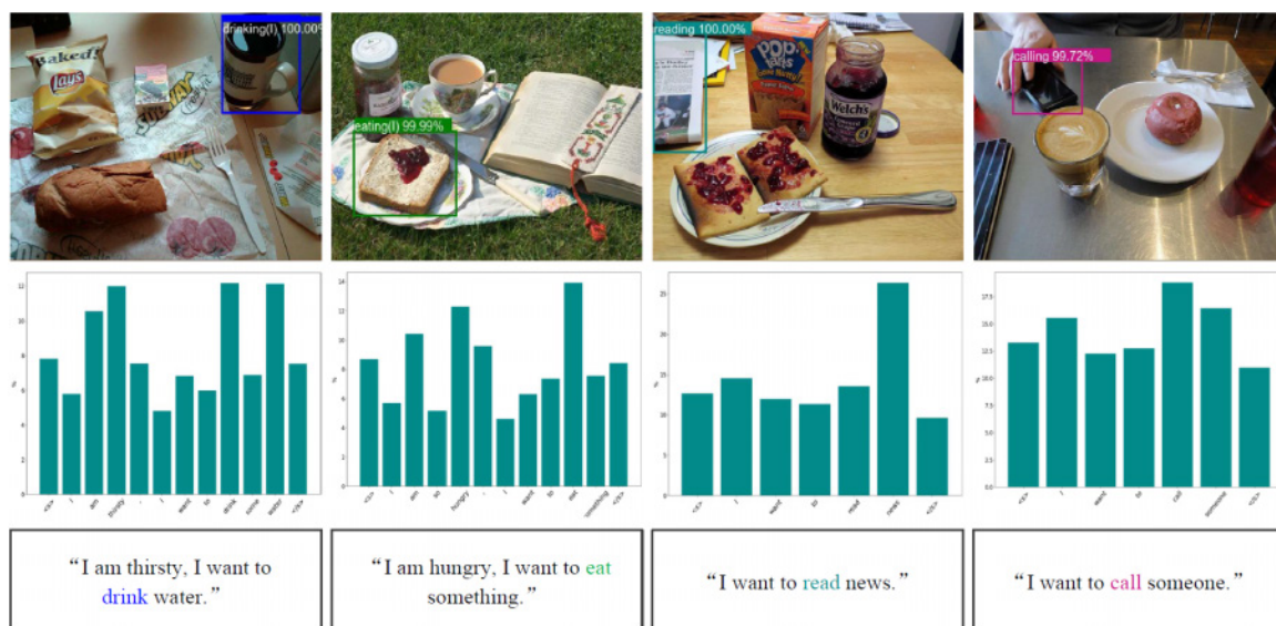
Figure 5.8: Example results of intention-related natural language query grounding via object affordance detection and intention semantic extraction. The first row lists example results of grounded target objects. The bar charts in the second row show the different weights of each word in given natural language instructions. The rectangles in the third row encompass the intention-related natural language queries, and the extracted intention semantics are covered with the related color with the detected affordances.
