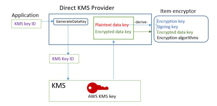
To generate encryption materials, the Direct KMS Provider asks AWS KMS to generate a unique data key for each item using an AWS KMS key that you specify. It derives encryption and signing keys for the item from the plaintext copy of the data key, and then returns the encryption and signing keys, along with the encrypted data key, which is stored in the material description attribute of the item.
