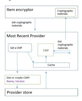
The Most Recent Provider saves versions of the CMPs that the provider store returns in a local Least Recently Used (LRU) cache in memory. The cache enables the Most Recent Provider to get the CMPs that it needs without calling the provider store for every item. You can clear the cache on demand.
