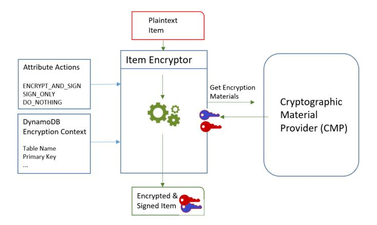
To encrypt and sign a table item, the DynamoDB Encryption Client needs:
