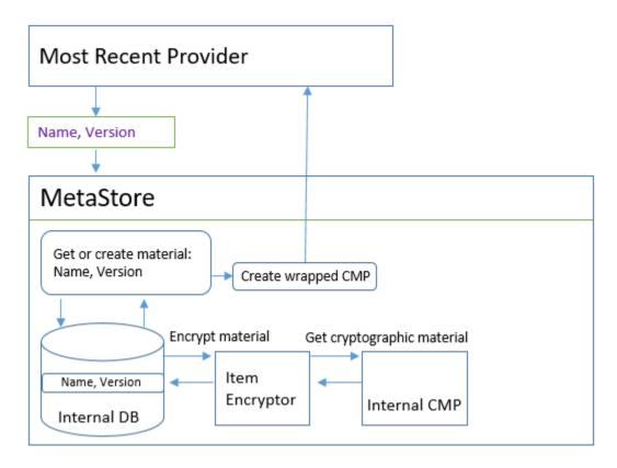
The MetaStore generates the Wrapped CMPs, and then stores them (in encrypted form) in an internal DynamoDB table. The partition key is the name of the Most Recent Provider material; the sort key its version number. The materials in the table are protected by an internal DynamoDB Encryption Client, including an item encryptor and internal <u>cryptographic materials provider</u> (CMP).
