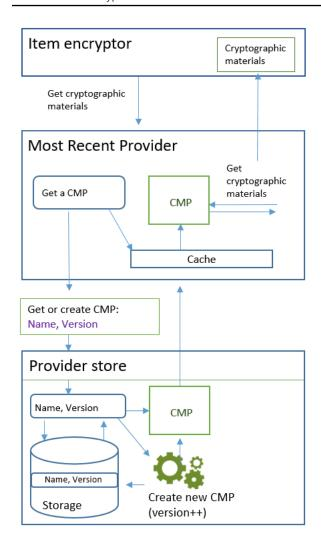
When you create a Most Recent Provider by using the <u>CachingMostRecentProvider symbol</u>, you specify a provider store, a name for the Most Recent Provider, and a <u>time-to-live</u> (TTL) value. You can also optionally specify a cache size, which determines the maximum number of cryptographic materials that can exist in the cache.
