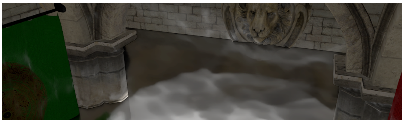
Figure 1: Ray-traced caustics in the flooded Sponza scene using only image-space computations. We achieve refractive caustics beneath the water, as well as reflective caustics on the wall and the ceiling without depending on hardware-accelerated ray tracing in recent GPUs.
