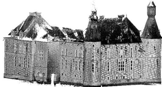
Figure 3: 3D reflectance only facade point cloud from the Trimble TX5 laserscanner (LPC)
