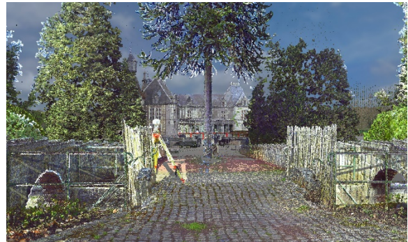
Figure 9: Zoom in-view from the parc combining all datasets with resolution-adapted LPC point cloud
