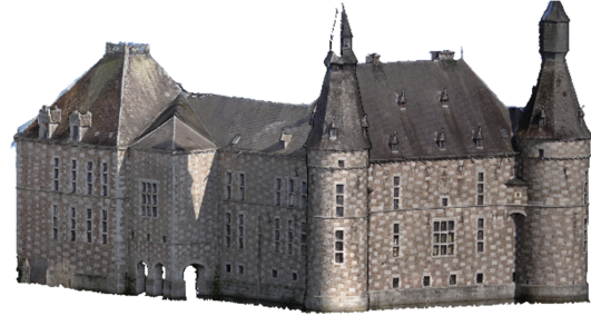
Figure 2: 3D coloured point cloud of the photogrammetric reconstruction (PPC)
