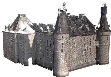
Figure 6: Point cloud from combining photogrammetric reconstruction and lasergrammetry acquisition
