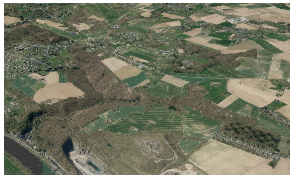
Figure 7: Colored LiDAR point cloud by combining orthophotos with LiDAR signal over zone of interest
