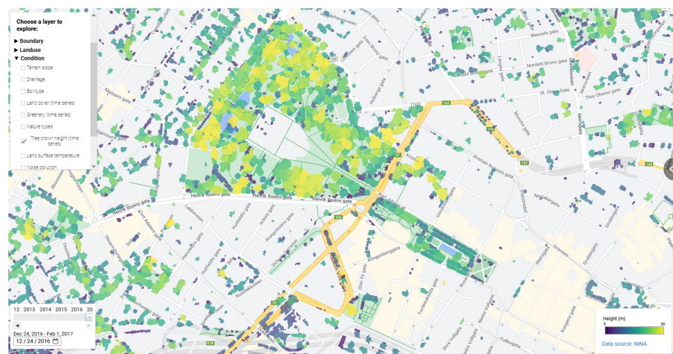
Figure 13.4 High-resolution thematic focus mapping of urban tree canopy asset extent and height (condition)
