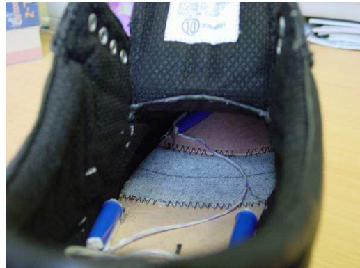
Figure 4: Vibrators installed in shoe
