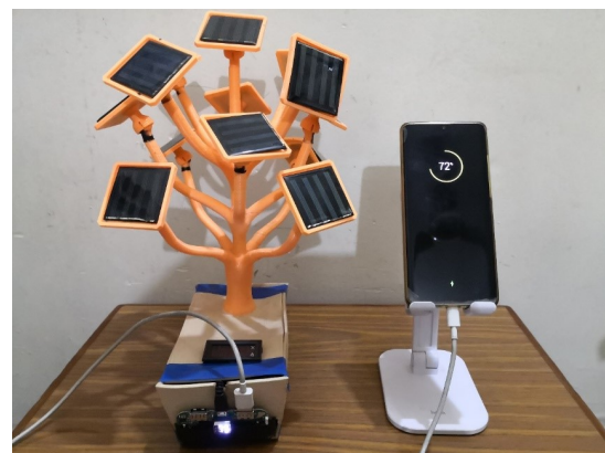
Figure 11: Charging the phone using the solar tree
