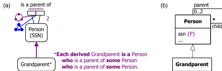
Fig. 5. In the ORM schema (a) the subtype Grandparent is semi-derived
