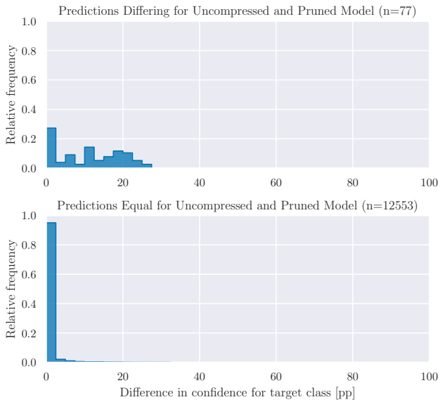
Figure 2: Difference (in percentage points) between the confidence in the target class for the uncompressed and pruned ResNet-18 trained on GTSRB. The upper plot shows the difference where the predictions of the both networks differ, the lower one where they are equal. In parenthesis we state the number of samples underlying the respective diagram, e.g., the n = 77 in the upper plot shows that for 77 samples the uncompressed and pruned model yielded a different classification result.
