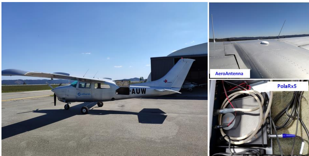
Figure 1: CESSNA C21A airplane (left), AeroAntenna (right top) and PolaRx5 (right down)
