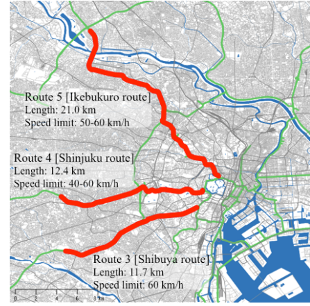
Figure 2: Three routes of Shuto Expressway within the Tokyo area
