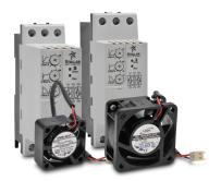
The SR22 series is a low-cost family perfect for use in applications where space is a concern. The SR22 soft starters use thyristors for controlled reduced voltage motor starting and stopping, then switch to internal bypass contacts for efficient running at rated speed. 3-potentiometer setup (Start Voltage, Start Time, and Stop Time) make installation and commissioning easy.
