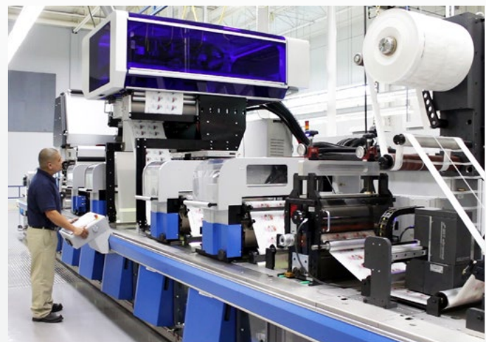
CCL Label hybrid digital and conventional printing with LED curing
