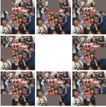
Figure 8: Eight different types of masking setting before predicting the people count in the central cell (red bounding box areas).
