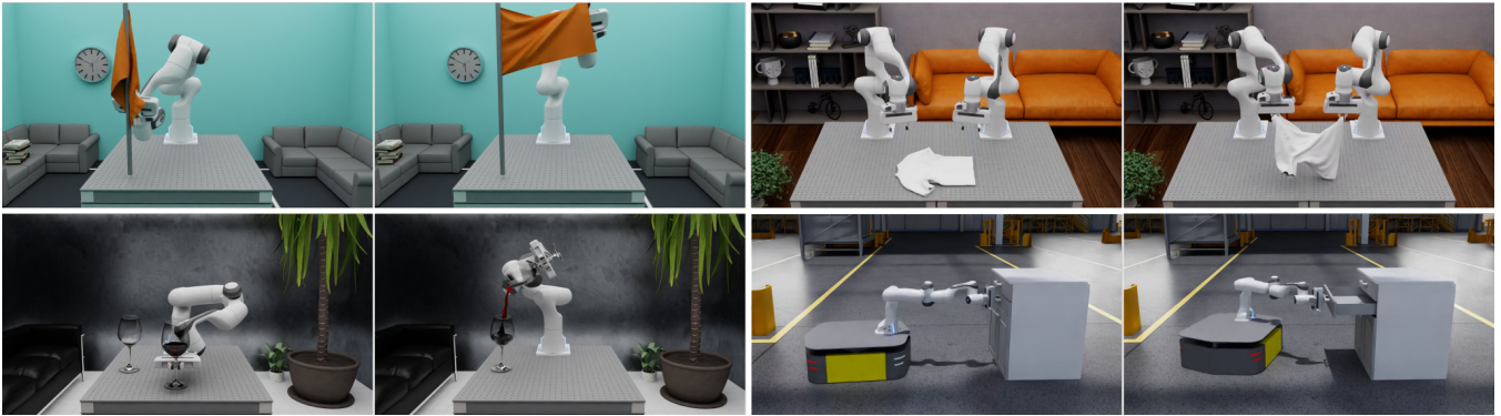
Fig. 6: Demonstration of the designed tasks using hand-crafted state machines and task-space controllers. Leveraging recent advances in physics engines, we support high-fidelity simulation of rigid and deformable objects. We include environments that allow switching between robots, objects, observations, and action spaces through configuration files ( videos ).
