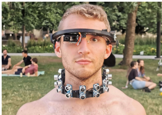
Fig. 1. 3D printed version of Vironment 3.0 with rigidly aligned sensors and OpenEyeTap computer vision and display system.
