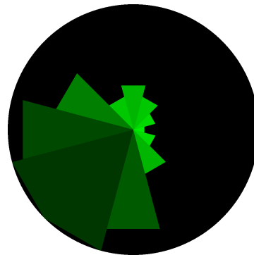
Fig. 8. The P.P.I. live user interface representing the social bubble around the user. The distance of the dodecant boundary to the center represents the distance of another individual to the wearer, at that specific location. The color is also modulated from black (infinite) to bright green (2cm) to represent the distance.
