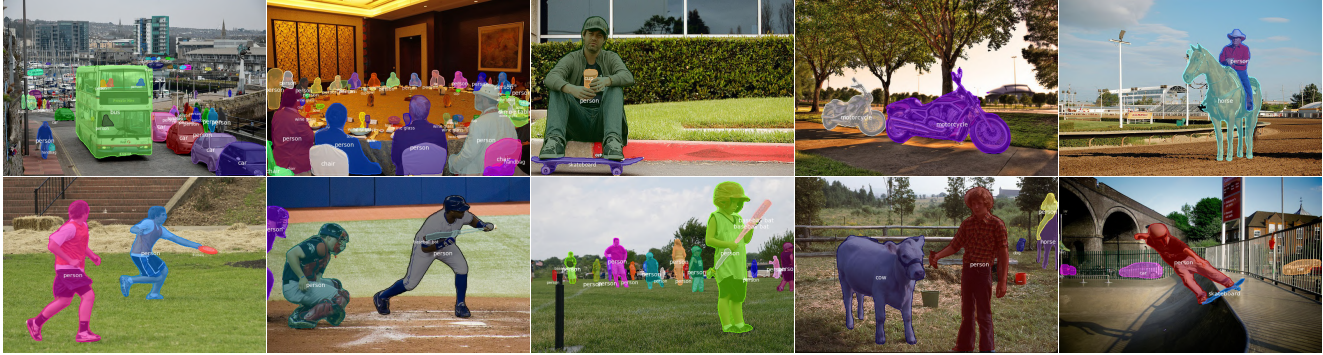
Figure 2: Results of CenterMask on COCO test set images. These results are based on Hourglass-104 backbone, achieving a mask AP of 34.5 and running at 12.3 fps. Our method differentiates objects well in overlapping conditions with precise masks.
