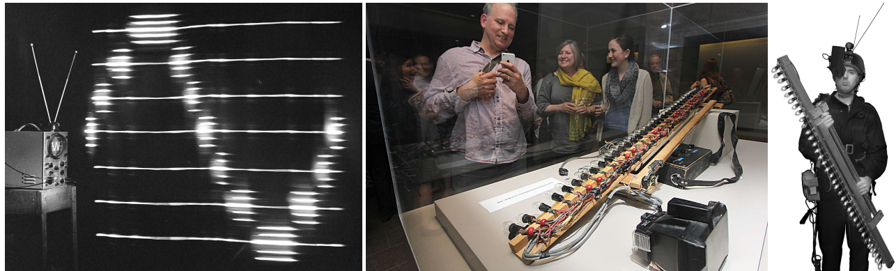
Figure 10: Early photograph of electromagnetic radio waves using the Sequential Wave Imprinting Machine (S. Mann, July 6, 1974, from Wikimedia Commons). Center: Sequential Wave Imprinting Machine exhibited at Smithsonian Institute and National Gallery, showing the linear array of 35 electric lights and the early wearable computer with lock-in amplifier and antenna sensor. Right: Early (1980) version of the apparatus with early wearable multimedia computer prototype.
