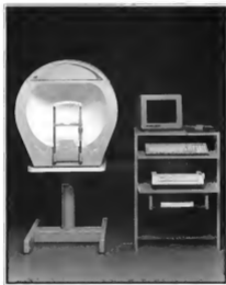
The Marco Technologies MT-336 Auto-Perimeter is a sophisticated ophthalmological measuring system built around an Atari 520ST. The program that runs the system was written in compiled GFA BASIC! You've come a long way, baby!
